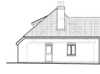
SIDE (WEST) ELEVATION THE BUNGALOW
